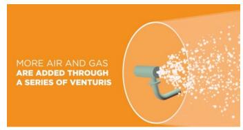
As the burning gases rapidly expand, more air and gas are added through a series of venturis
